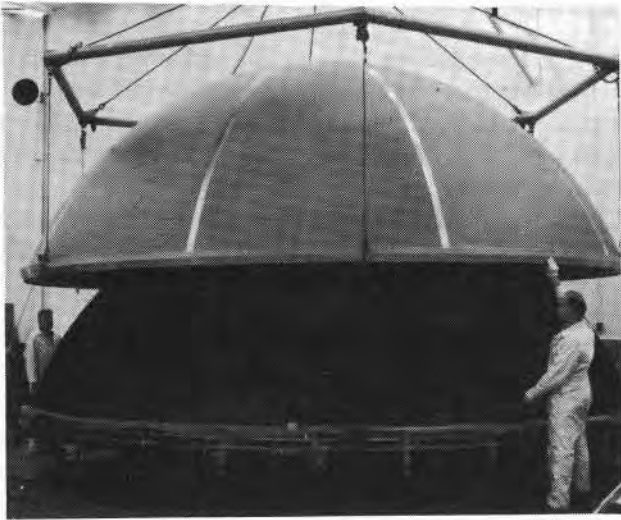
Fig. 11 - Bonding forward and aft faces of common bulkhead
