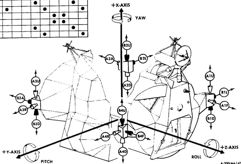
Figure 2.4-9. Reaction Control Subsystem - Thruster-On Failure Correction
