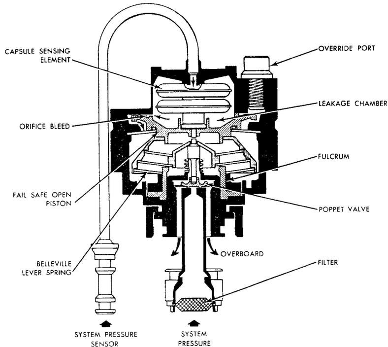
Figure 2.6-17. Overboard Relief Valve - Functional Schematic
