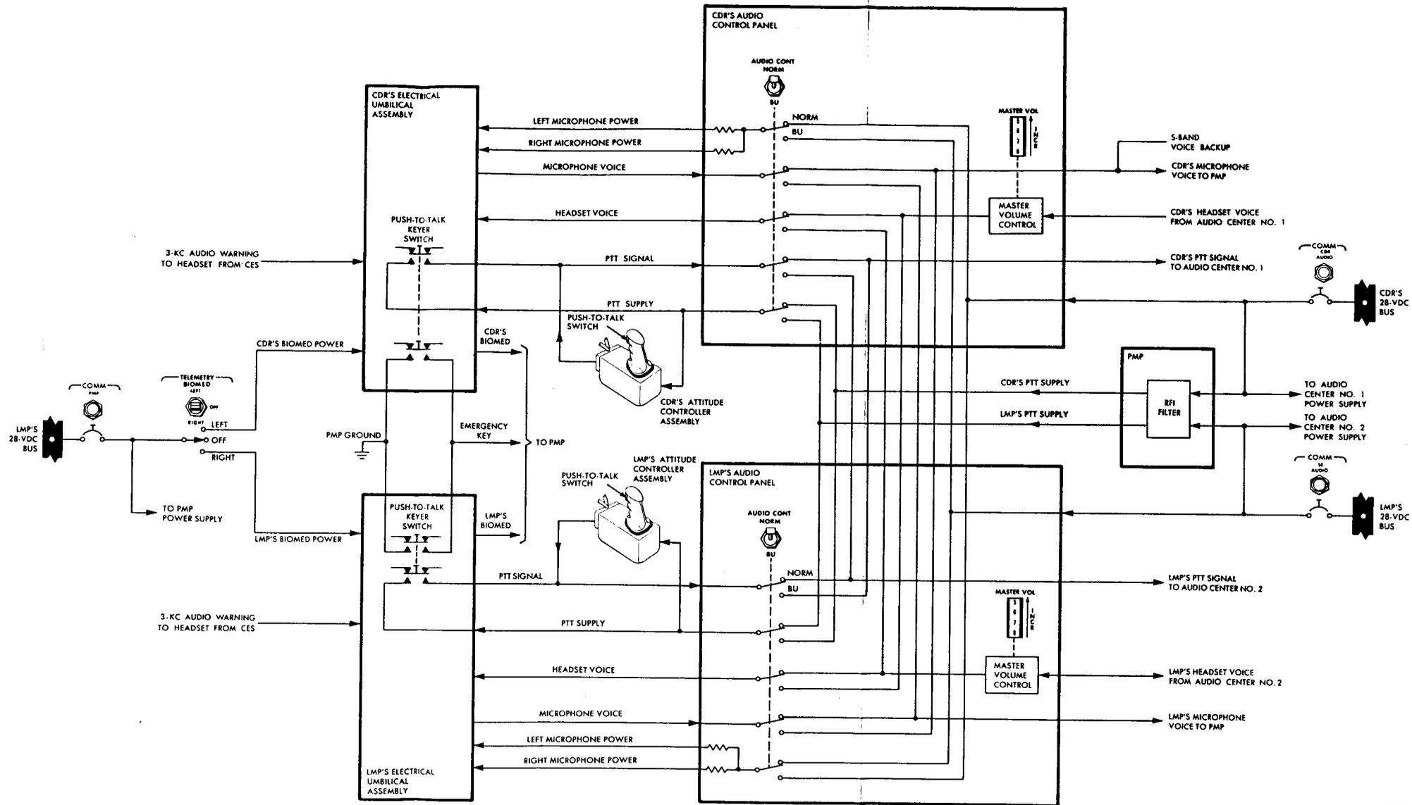
Figure 2-7-16. Audio Control Circuits - Simplified Block Diagram
