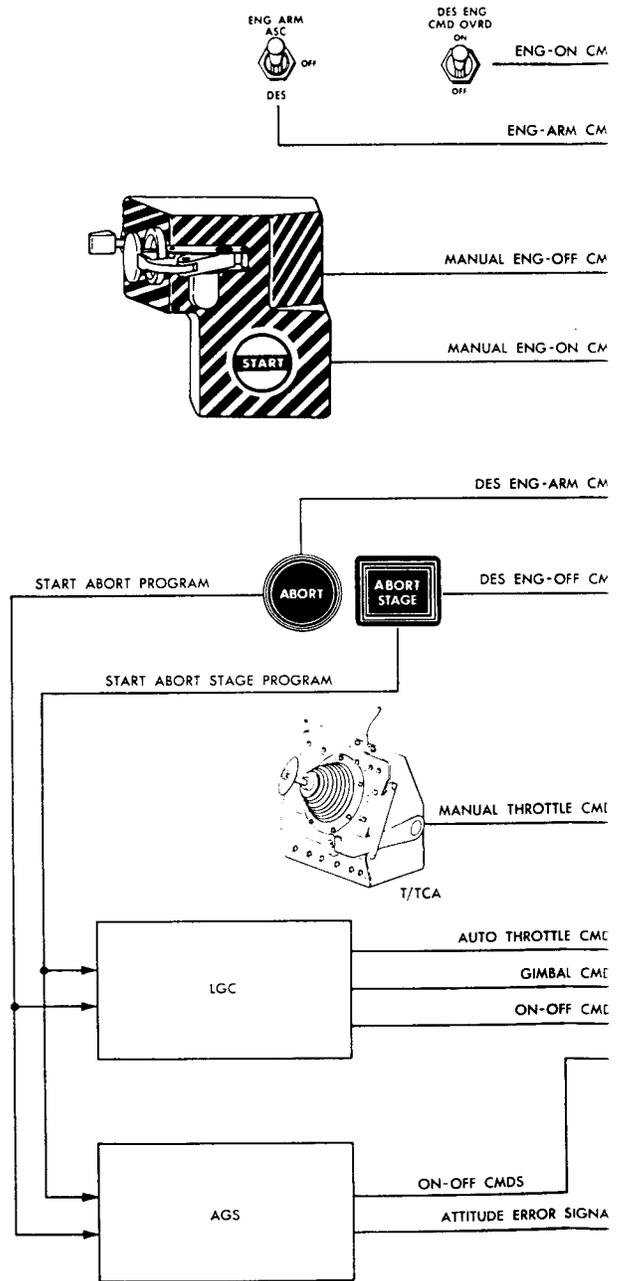
analog output of the DECA controls descent engine thrust. In the automatic mode, the thrust/translation controller assemblies (TTCA's) can be used by the astronauts to increase descent engine throttle (overriding the automatic throttle command); the TTCA's cannot be used, however, to decrease the throttle command. (Refer to paragraph 2.3.3.3.1.) In the manual throttle mode, the astronauts have complete control over descent engine thrust.
