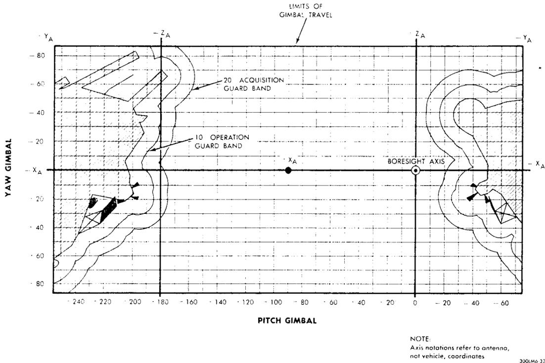
Figure 2.7-24. S-Band Steerable Antenna - Vehicle Blockage Diagram
