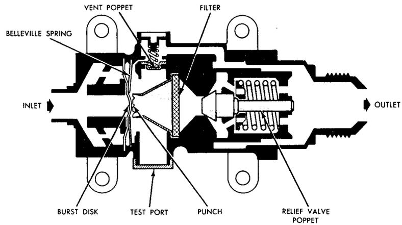
Figure 2.4-11. Relief Valve Assembly
