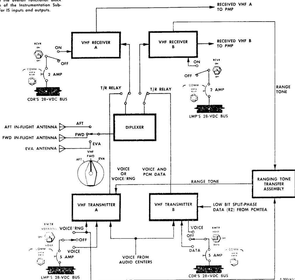
Figure 2.7-9. VHF Equipment - Block Diagram
