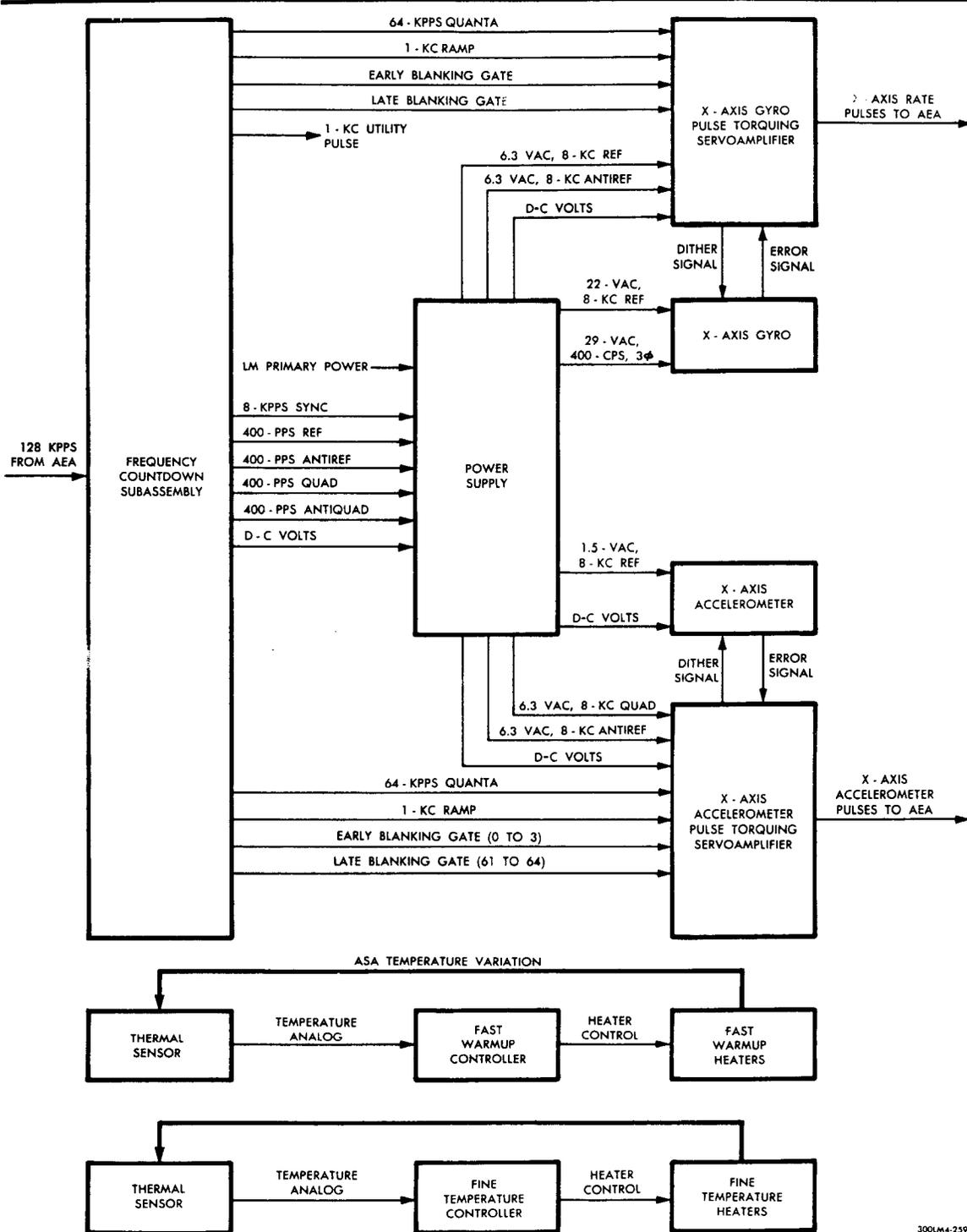
Figure 2.1-34. Abort Sensor Assembly - Block Diagram
