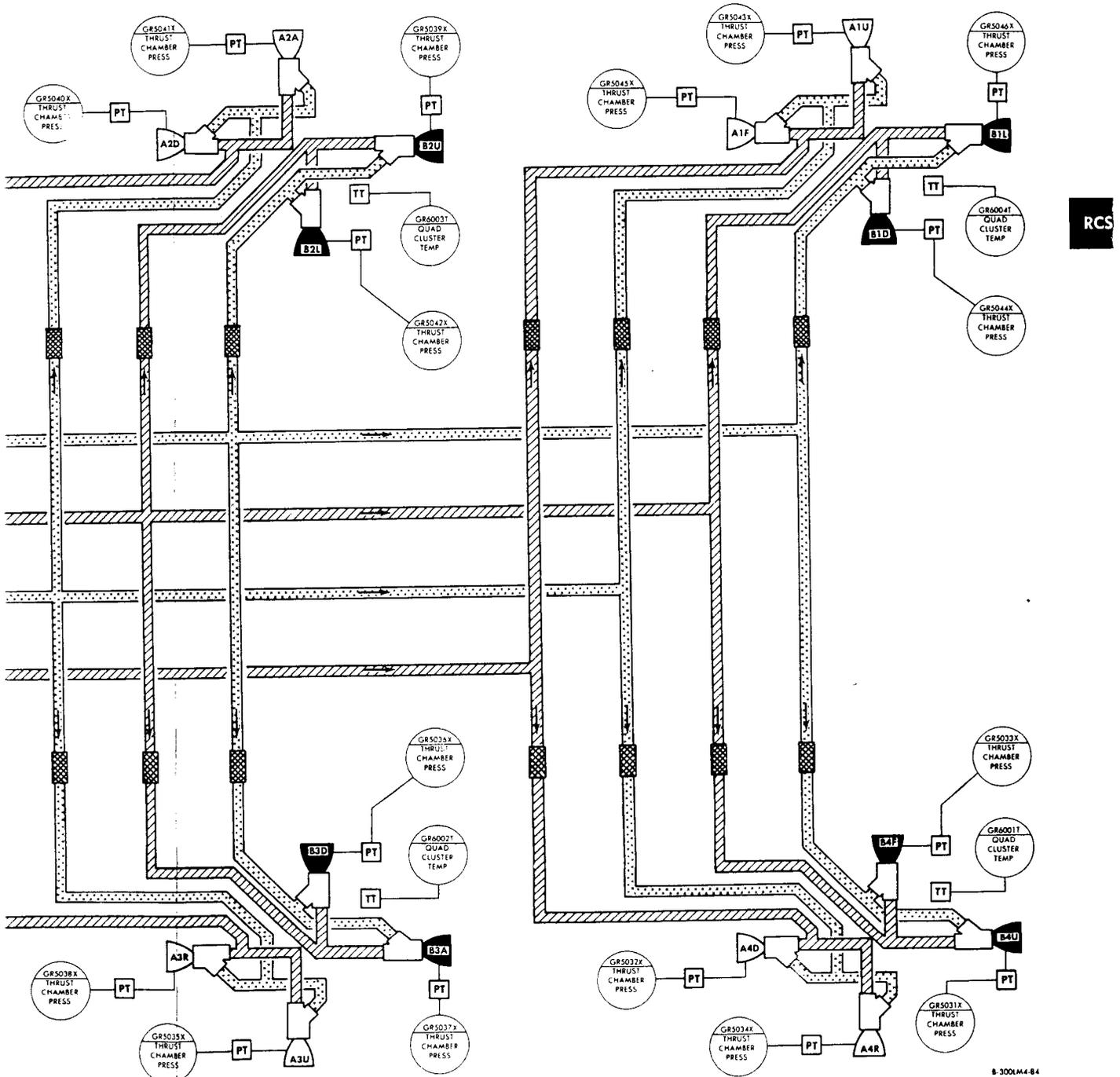
Figure 2.4-13. Reaction Control Subsystem - Telemetry Points
