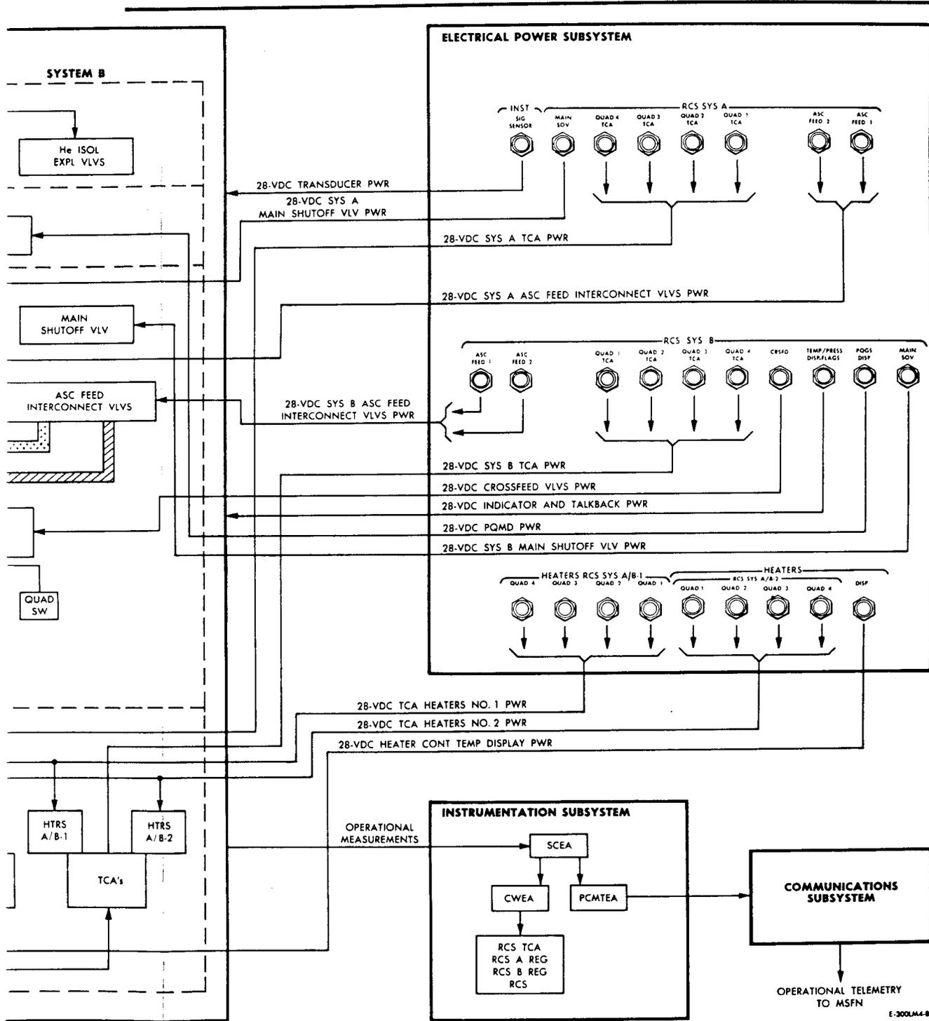
Figure 2.4-2. Reaction Control Subsystem - Interface Diagram
