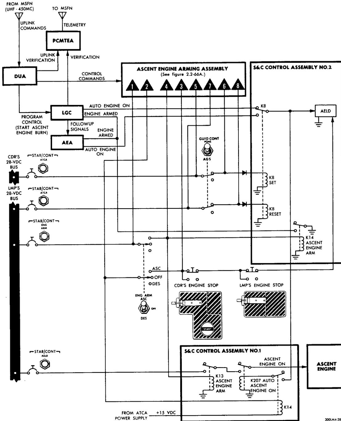
Figure 2.1-54. Ascent Engine Arming Assembly - Functional Diagram
