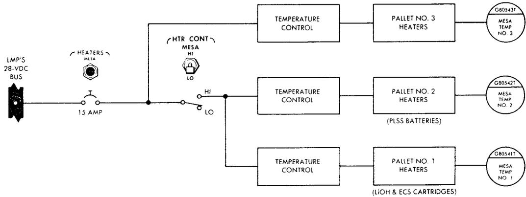
Figure 2.11-17. Modularized Equipment Stowage Assembly Heater Circuits
