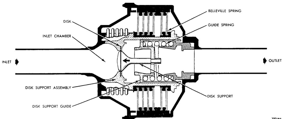
Figure 2.3-11. Descent Propulsion Section - Burst Disk Assembly
