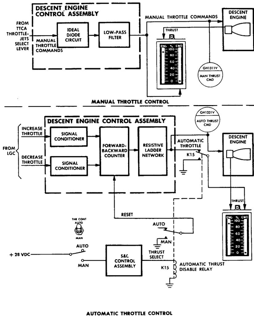
Figure 2.1-49. Descent Engine Control Assembly - Throttle Control Diagram
