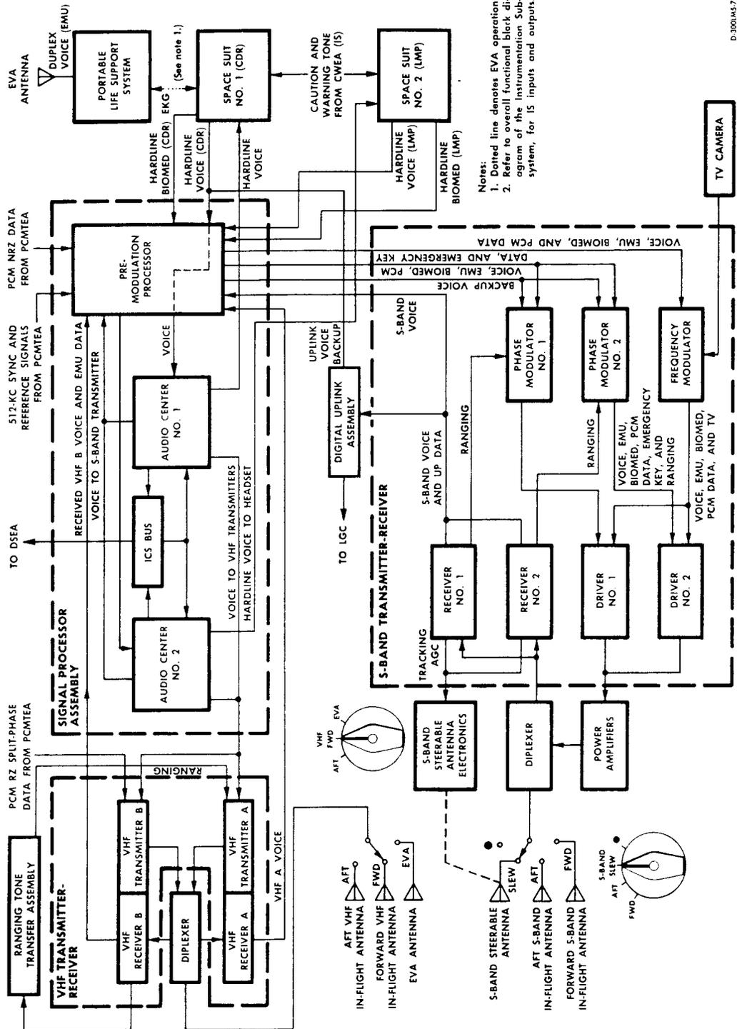
Figure 2.7-2. Communications Subsystem - Simplified Block Diagram
