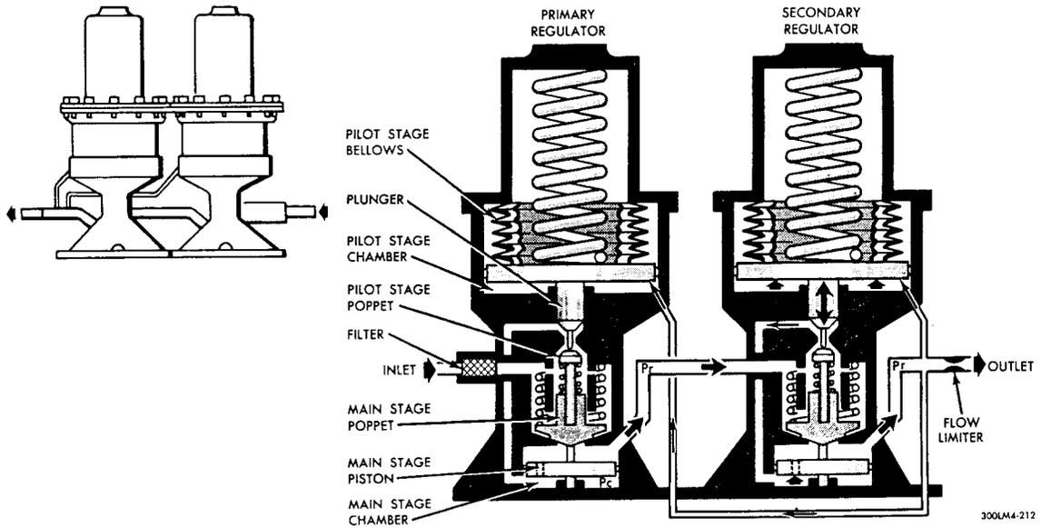
Figure 2.4-10. Helium Pressure Regulator Assembly
