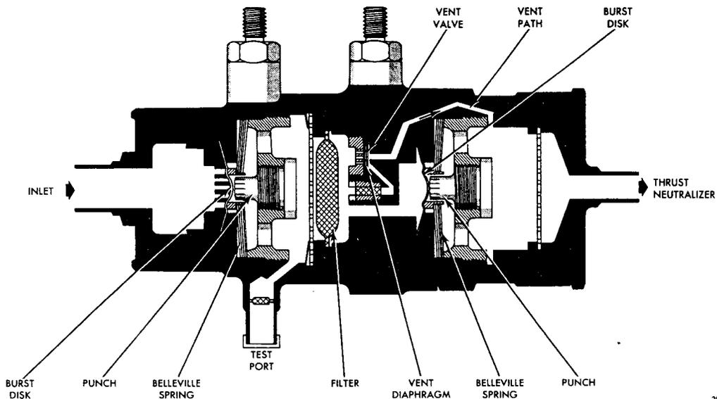
Figure 2.3-7A. Cryogenic Helium Storage Vessel - Burst Disk Assembly
