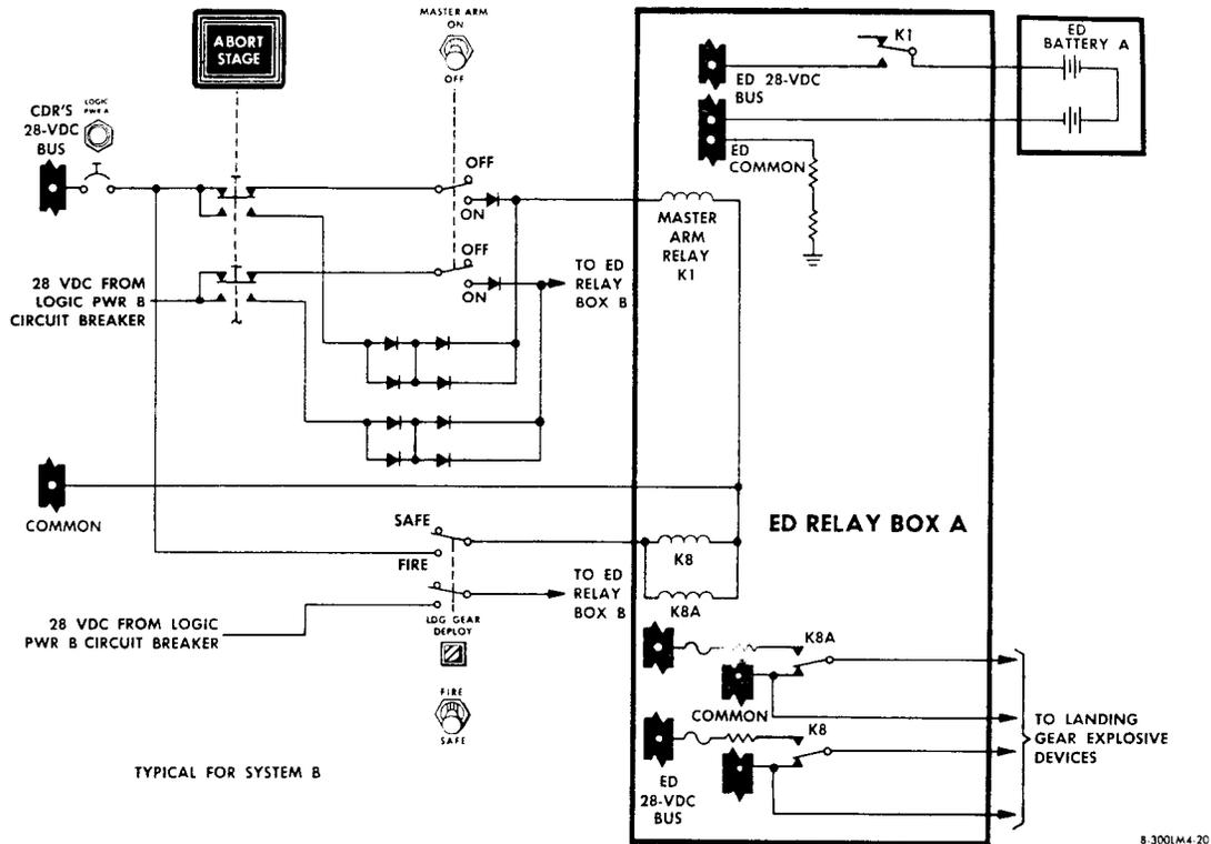
Figure 2.8-6. Landing Gear Deployment - Simplified Schematic Diagram
