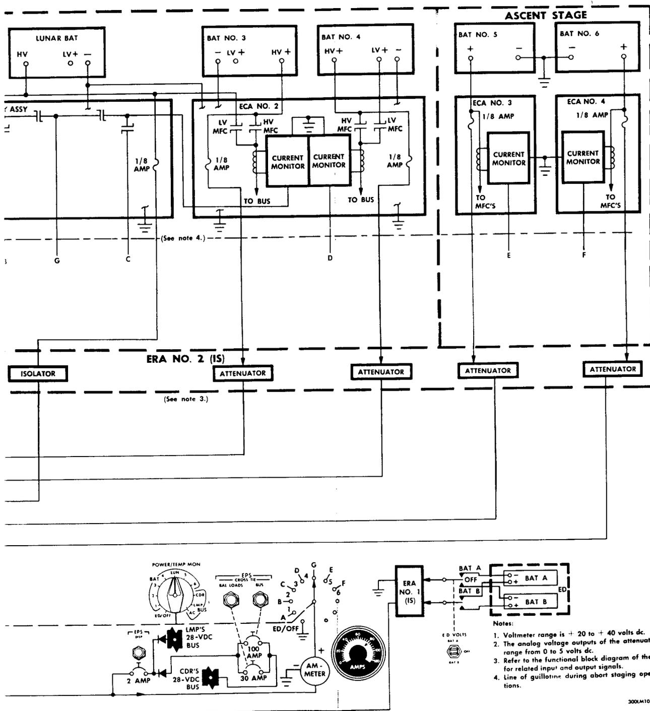
Figure 2.5-7. Battery Voltage- and Current-Monitoring Circuits - Simplified Diagram
