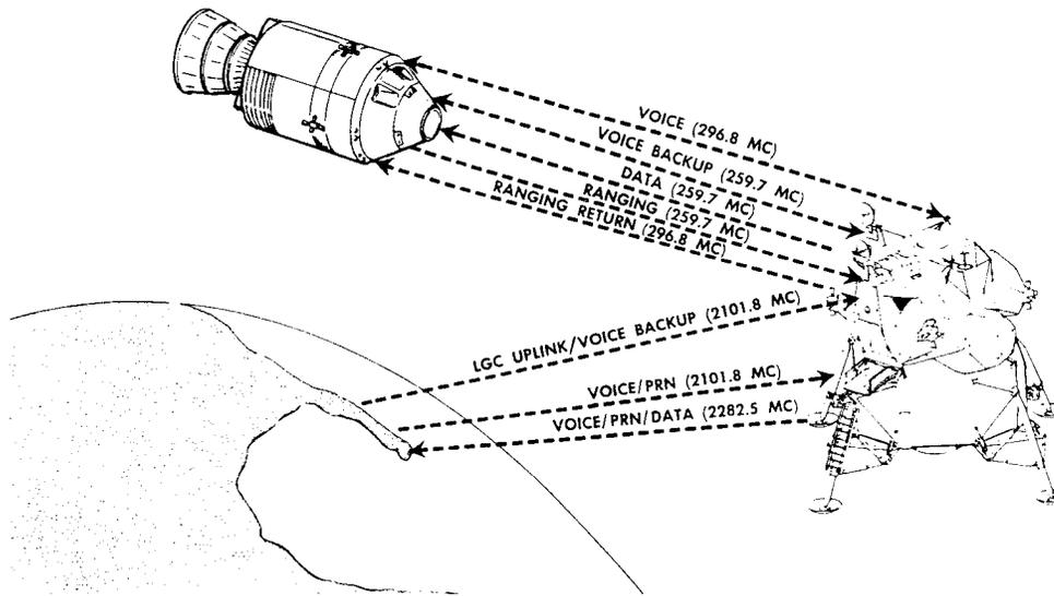
Figure 2.7-4. In-Flight Communications
