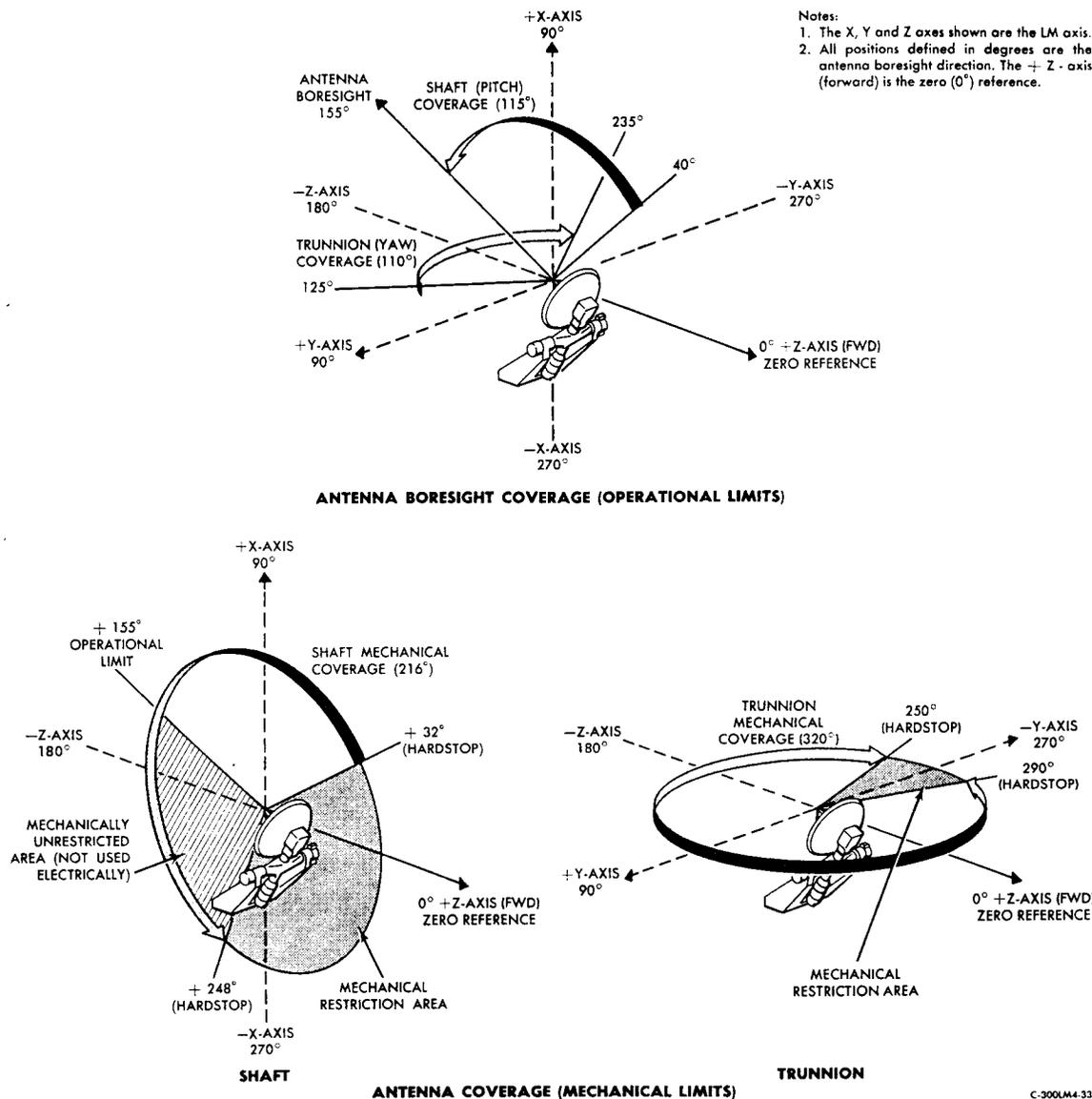
Figure 2.2-6. Rendezvous Radar - Antenna Orientation No. II
