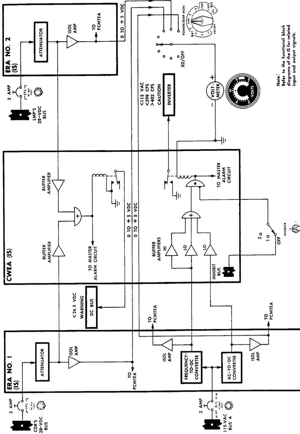
Figure 2.5-8. Primary Bus Voltage-Monitoring Circuits - Simplified Schematic Diagram
