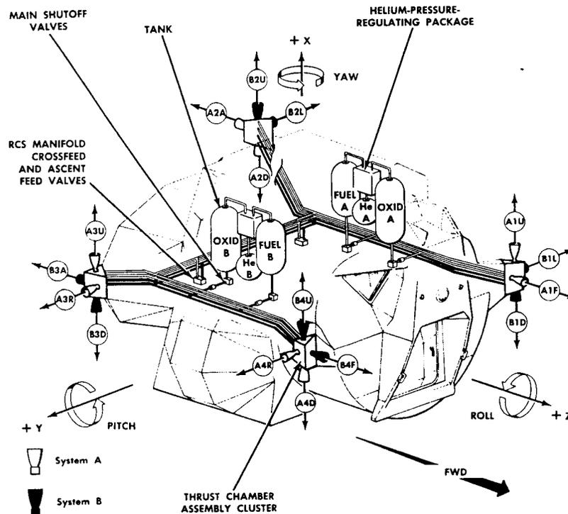
Figure 2.4-1. Reaction Control Subsystem - Component Location
