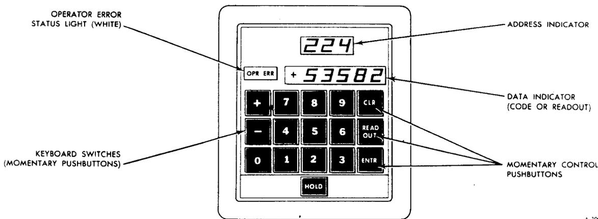
Figure 2.1-7. Data Entry and Display Assembly - Pictorial
