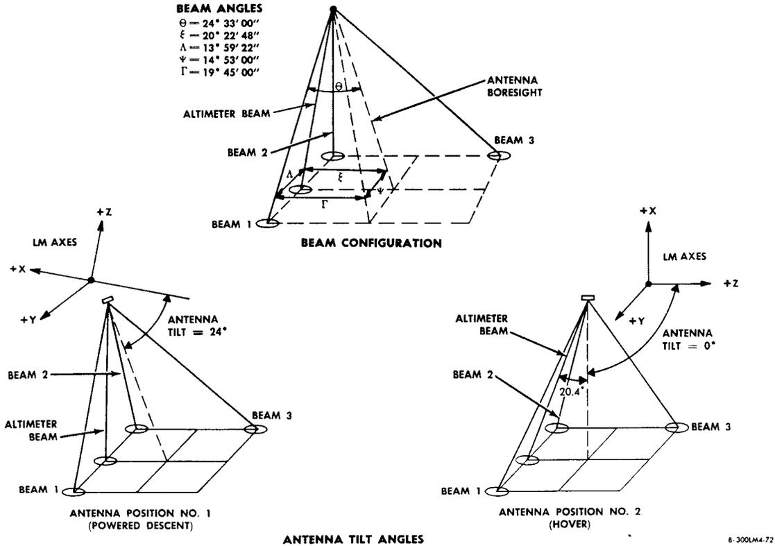
Figure 2.2-12. Landing Radar - Antenna Beam Configuration
