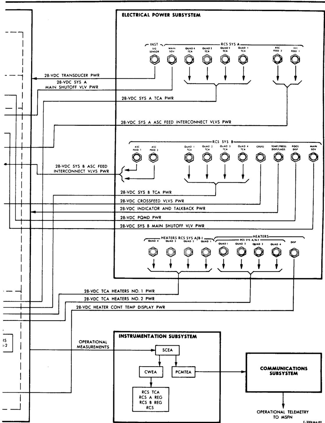
Figure 2.4-2. Reaction Control Subsystem - Interface Diagram
