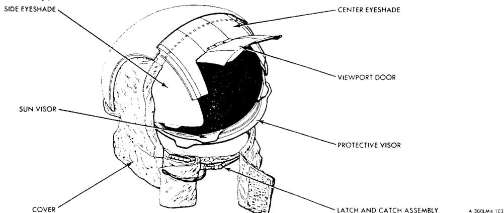
Figure 2.11-4. Lunar Extravehicular Visor Assembly
