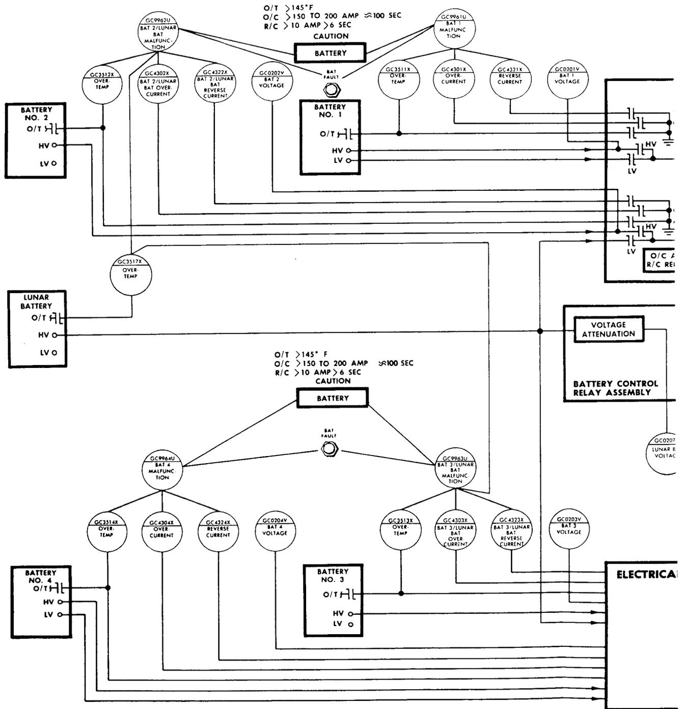
Figure 2.5-4. Descent Power Distribution - Functional Block Diagram
