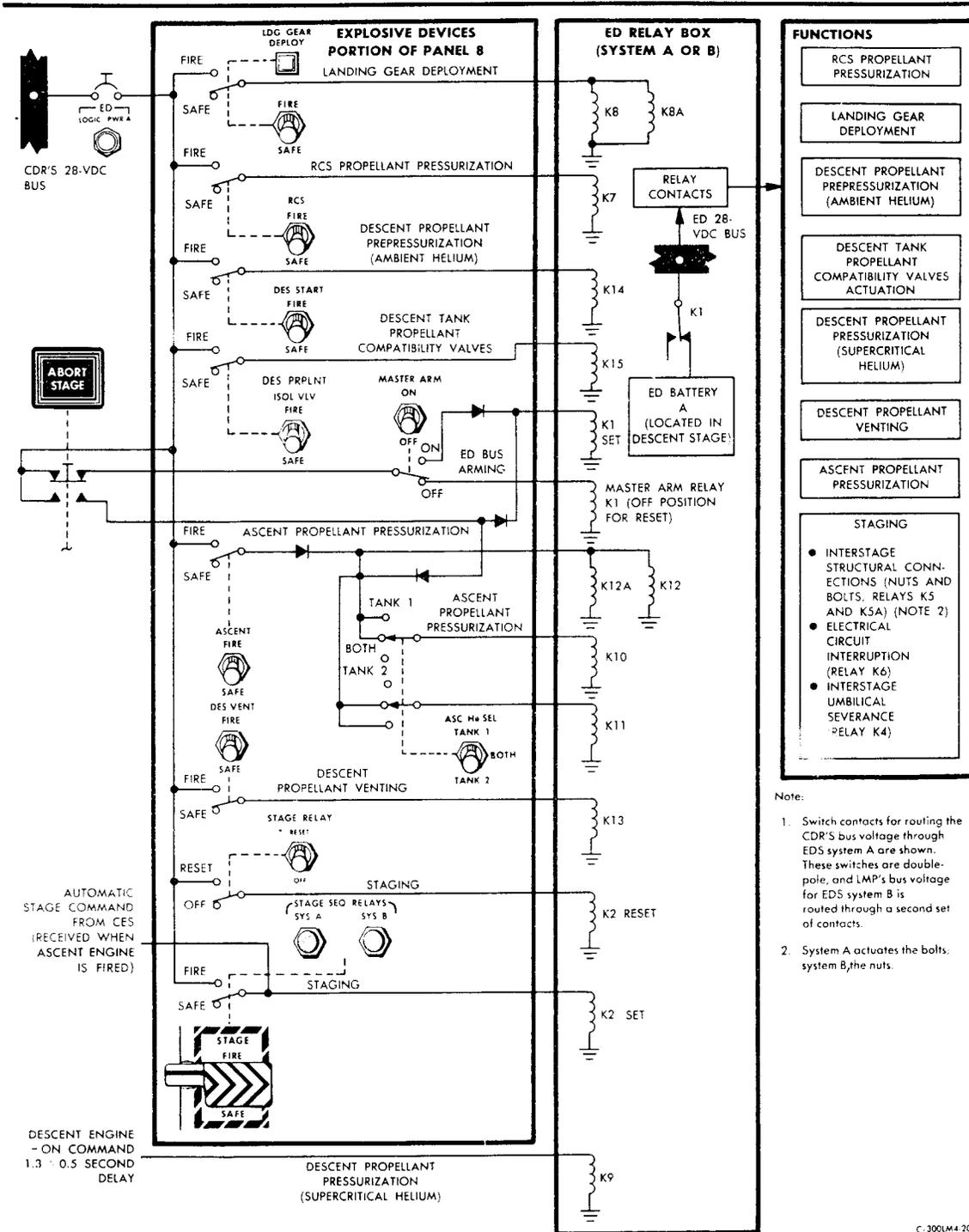
Figure 2.8-3. Explosive Devices Subsystem - Overall Functional Diagram
