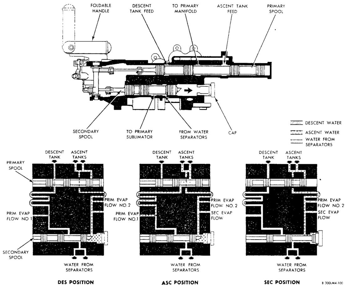
Figure 2.6-22. Water Tank Selector Valve - Functional Schematic
