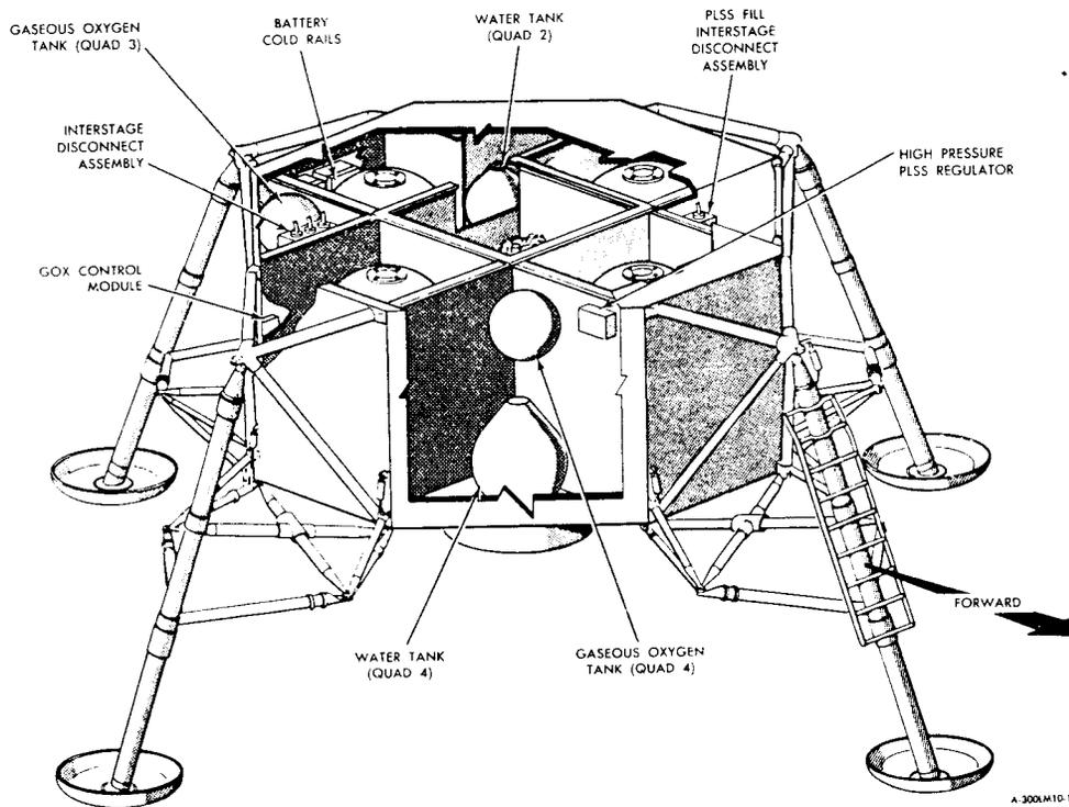
Figure 2.6-1. Environmental Control Subsystem - Component Location (Sheet 1 of 3)
