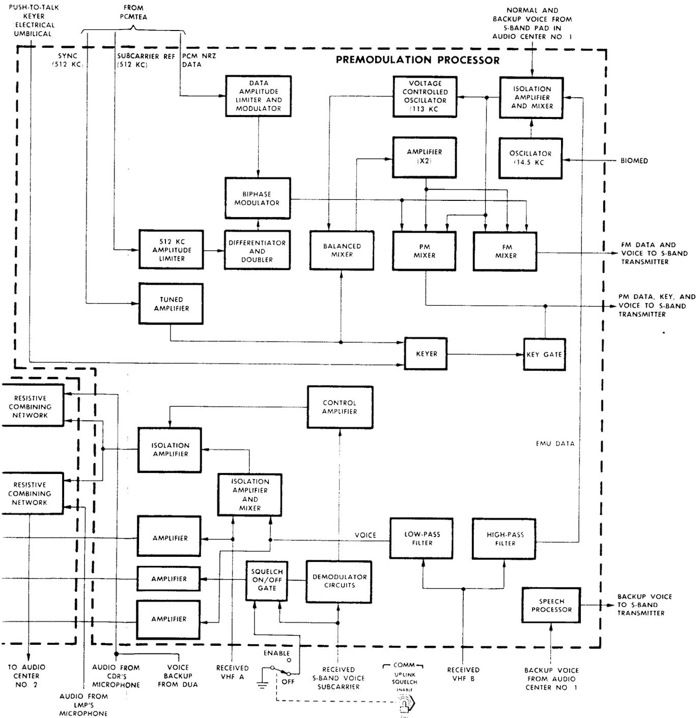
Figure 2.7-13. Signal Processor Assembly - Block Diagram
