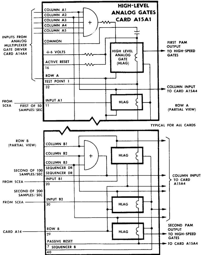
Figure 2.9-6. High-Level Analog Multiplexer Card - Simplified Logic Diagram
