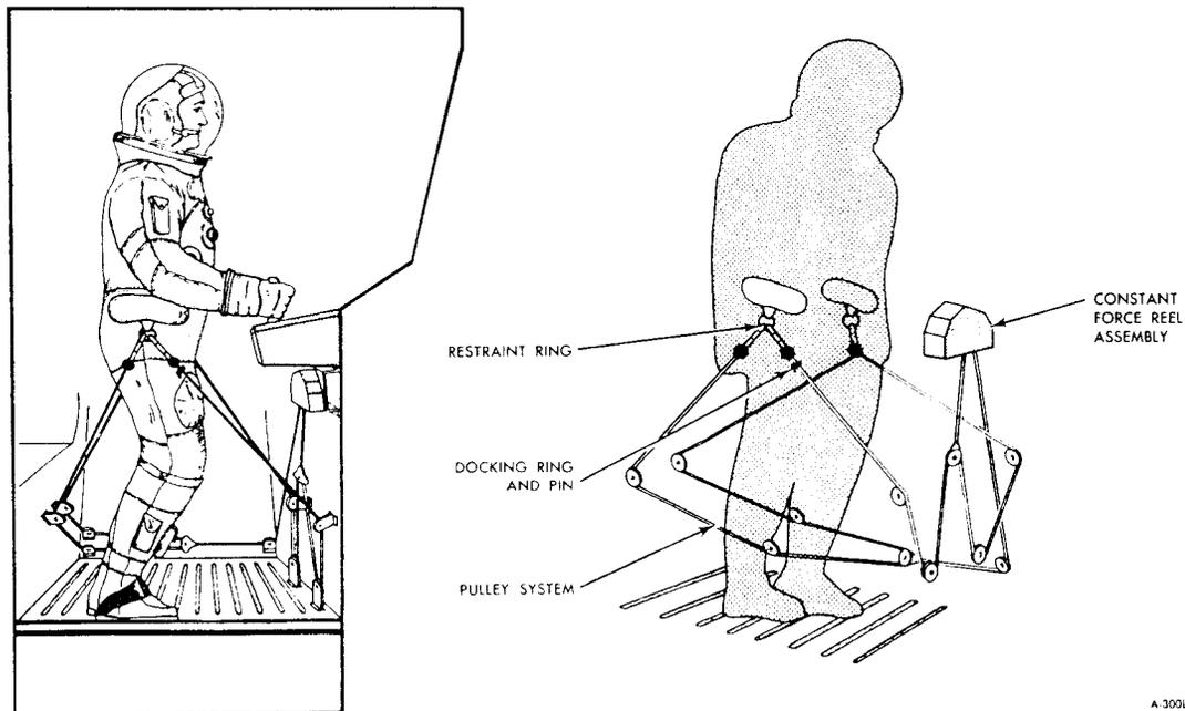
Figure 2.11-10. Restraint Equipment
