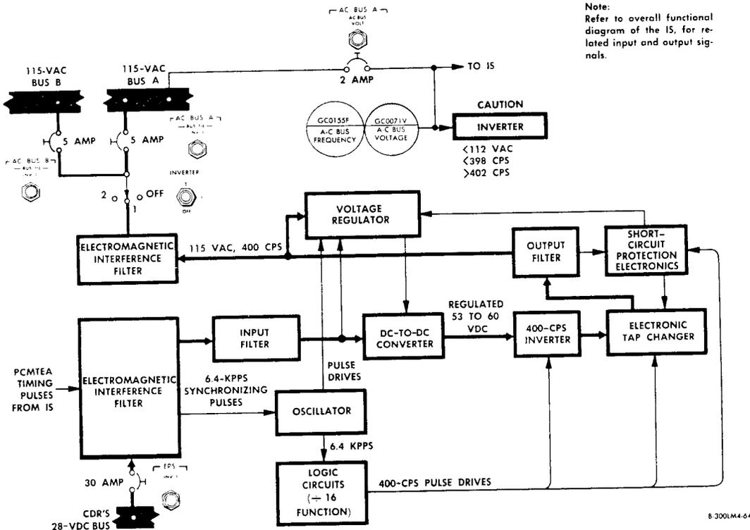
Figure 2.5-15. Inverter No. 1 - Block Diagram
