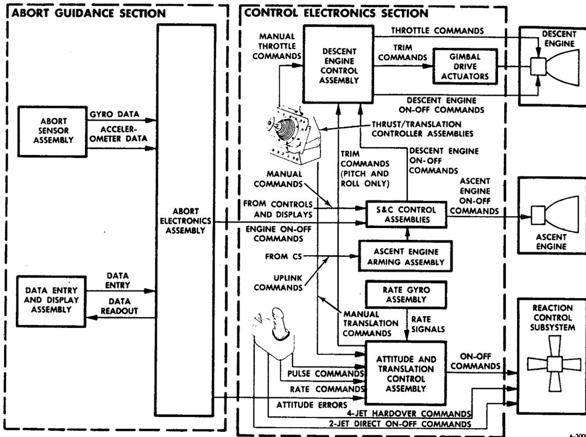
Figure 2.1-14. Abort Guidance Path - Simplified Block Diagram
