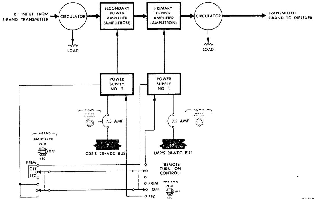
Figure 2.7-8. S-Band Power Amplifier - Block Diagram
