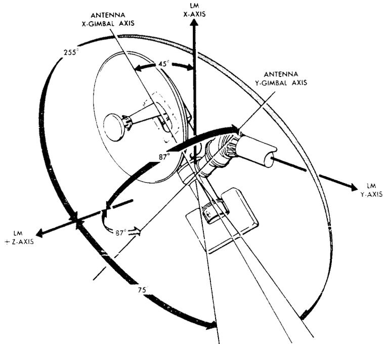
Figure 2.7-23. S-Band Steerable Antenna - Antenna Gimballing
