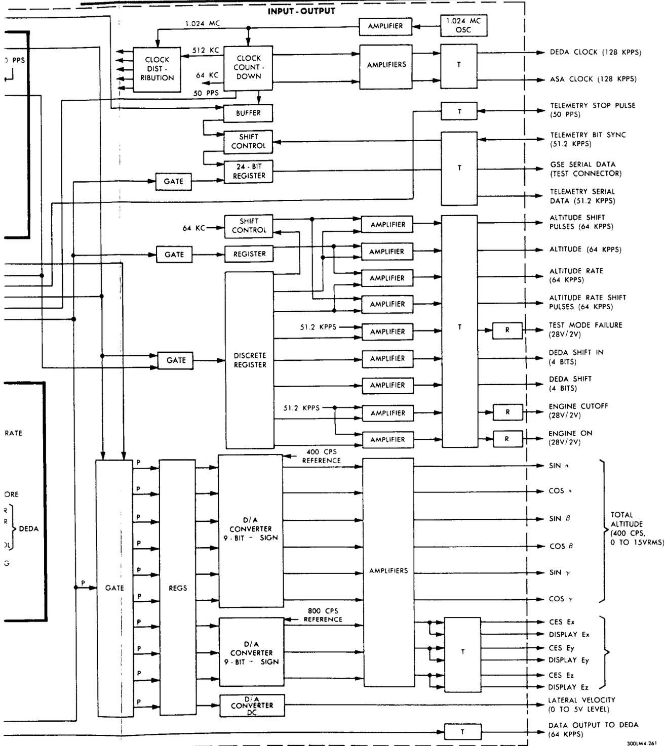
Figure 2.1-36. Abort Electronics Assembly - Detailed Block Diagram
