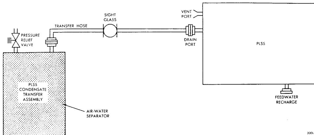
Figure 2.11-8. PLSS Condensate Transfer - Schematic Diagram
