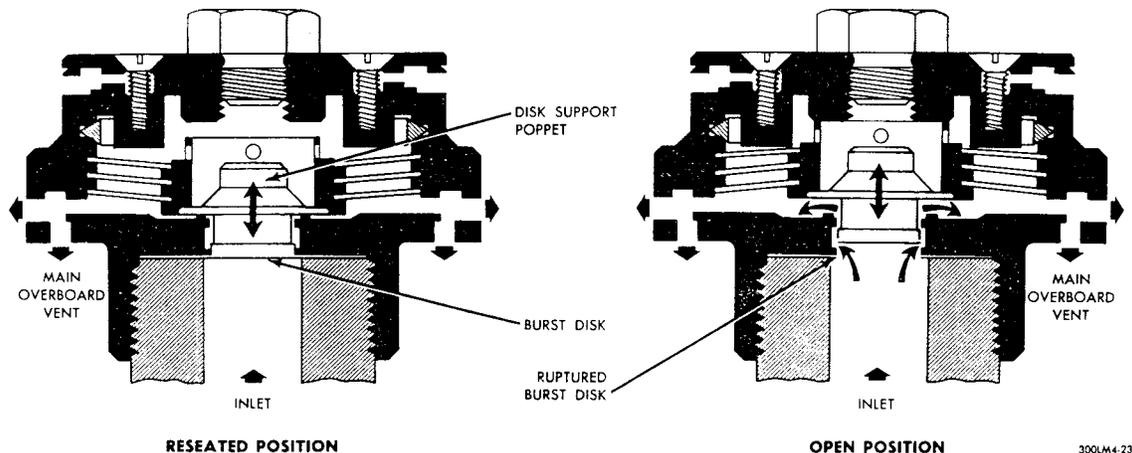
Figure 2.6-18. Burst Diaphragm Assembly - Functional Schematic
