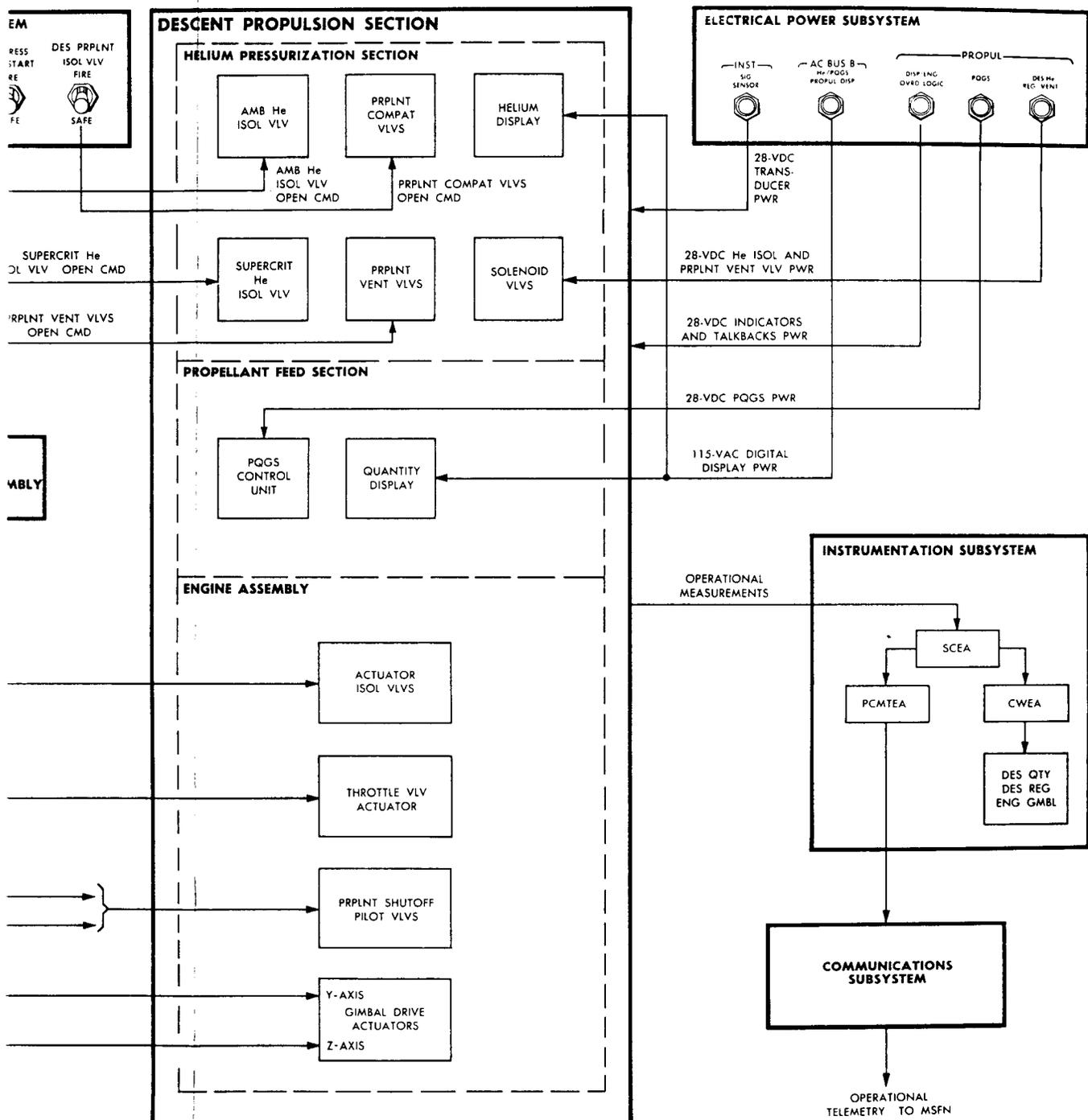
Figure 2.3-2. Descent Propulsion Section - Interface Diagram
