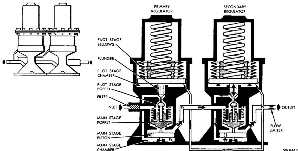
Figure 2.3-21. Ascent Propulsion Section - Helium Pressure Regulator Assembly
