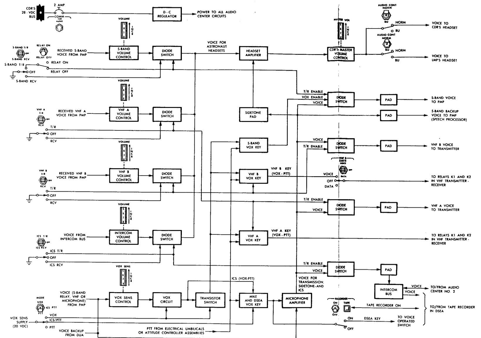
Figure 2.7-15. Audio Center No. 1 - Block Diagram
