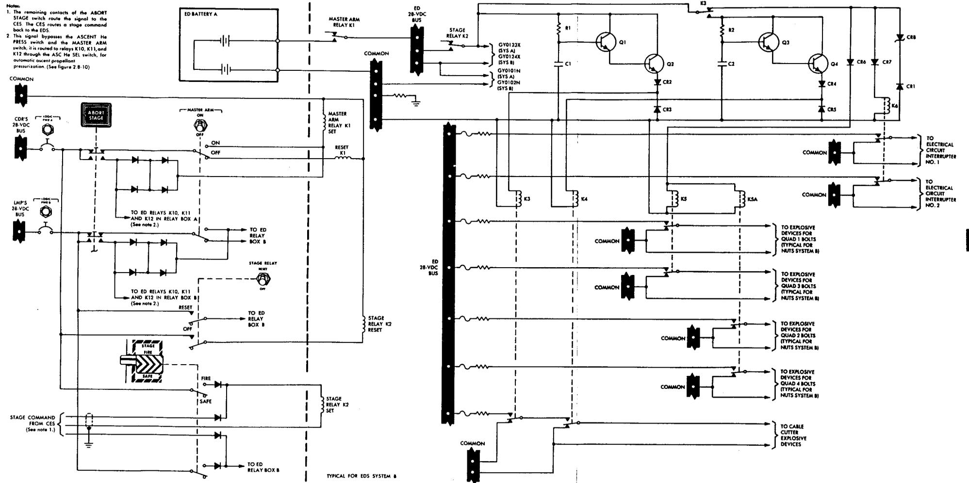
Figure 2.8-9. Stage Sequence - Simplified Schematic Diagram
