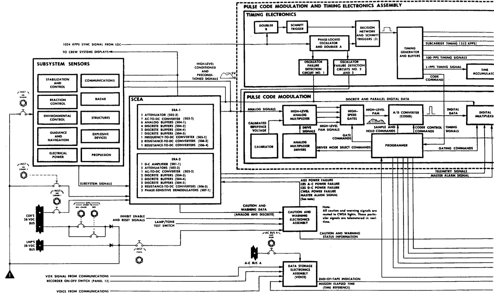
Figure 2.9-2. Instrumentation Subsystem - Overall Functional Block Diagram
