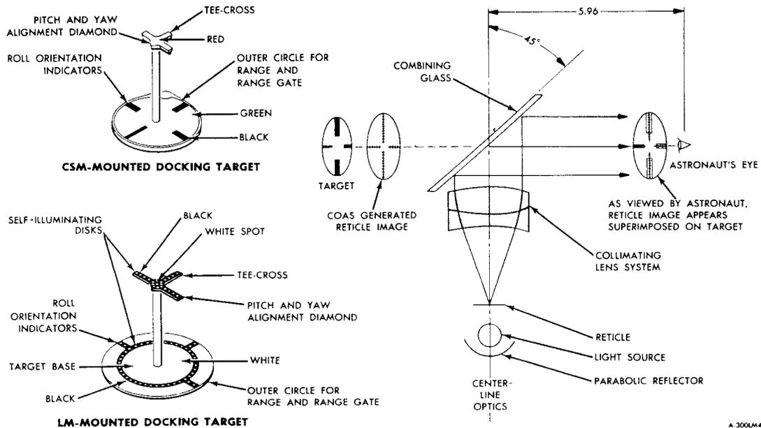
Figure 2.11-12. COAS Functional Schematic and Docking Targets
