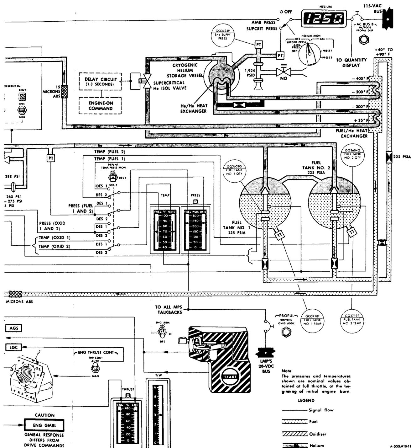
Figure 2.3-3. Descent Propulsion Section - Simplified Functional Flow Diagram
