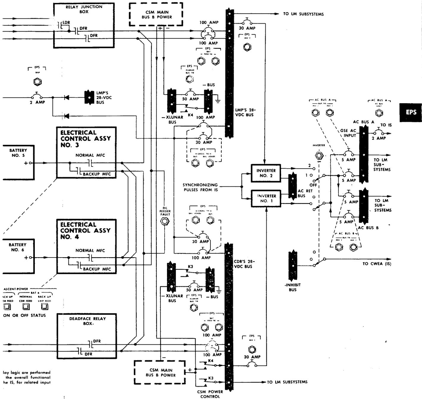
Figure 2.5-3. Electrical Power Subsystem - Functional Flow Diagram
