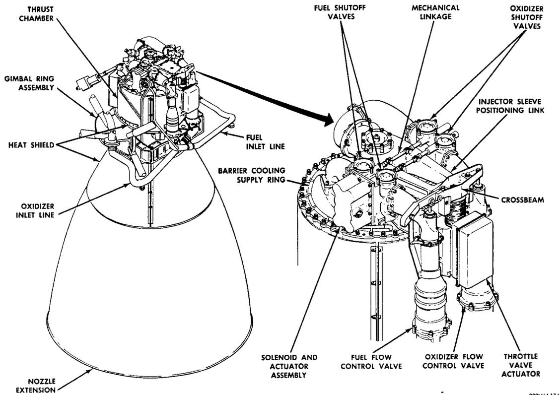
Figure 2.3-6. Descent Engine and Head End Assembly
