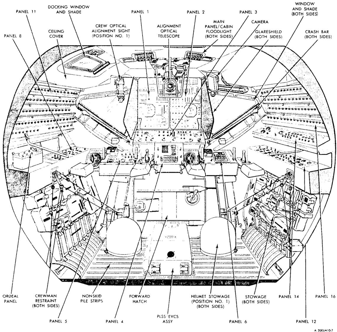
Figure 2.11-18. LM Cabin Interior, Forward View
