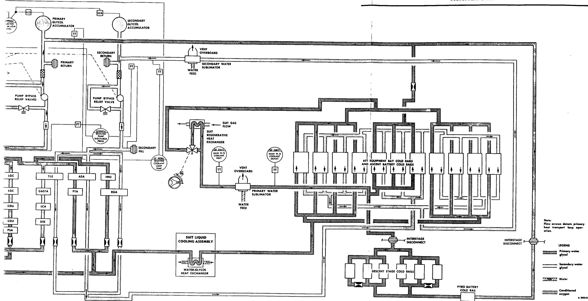
Figure 2.6-9. Heat Transport Section - Simplified Functional Flow Diagram
