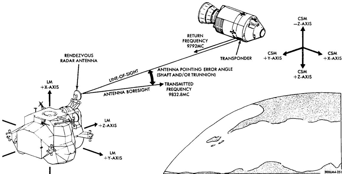
Figure 2.2-1. LM Rendezvous Radar and CSM Target Orientation
