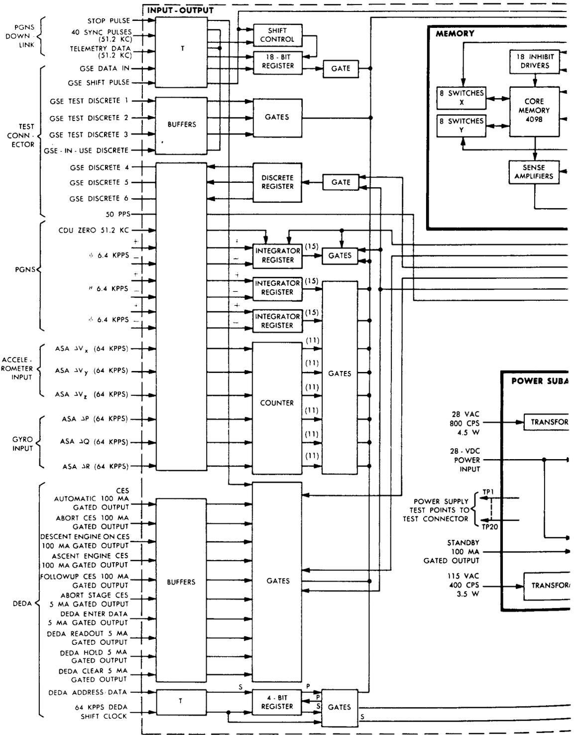
**Cycle Counter.** The cycle counter is a five-bit counter that controls shift instructions and certain long orders. The counter is loaded from the six least significant bits of the M-register.
